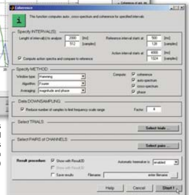
coherence analysis for predefined pairs of channels (and comparison with significance test)
